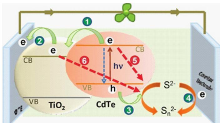
**Figure 1:** Schematic diagram of the working mechanism of SSSCs [3].
