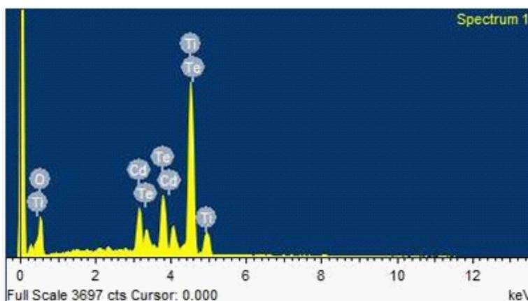
**Figure 4:** Typical EDX spectrum of FTO/TiO<sub>2</sub>/CdTe nanoarray thin films.
