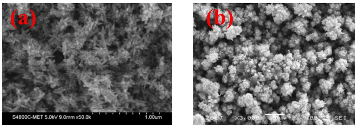
**Figure 3:** Scanning Electron Microscopy (SEM) images of (a) FTO/TiO<sub>2</sub> and (b) FTO/TiO<sub>2</sub>/CdTe nanoarray thin films.
