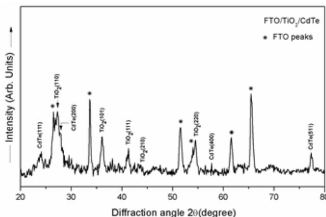
**Figure 2:** XRD pattern of FTO/TiO<sub>2</sub>/CdTe nanocomposite (peaks of FTO glass substrate are marked by stars)
